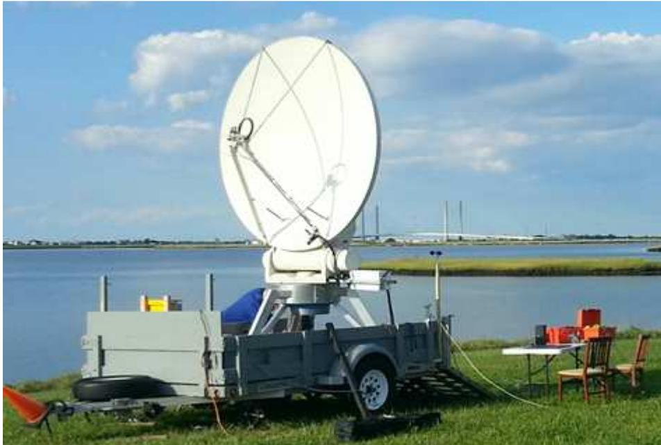
Photo 2: WA3LBI's portable 2.2 metre dish on location
