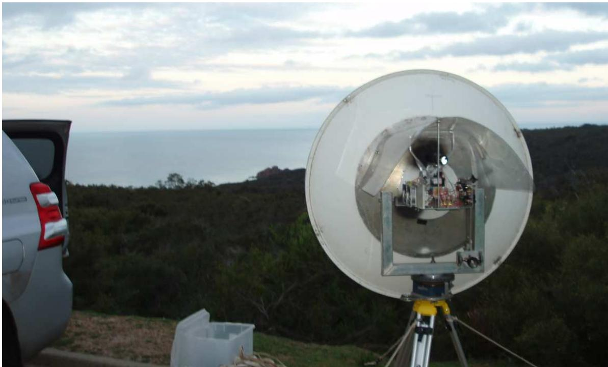
Photo 1: VK7MO's 1.13 metre dish set up at Meelup beaming across the water
