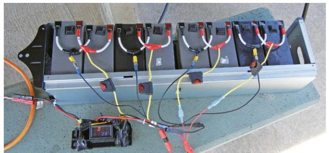
W5RZ's bank of 7.2 A/h sealed lead-acid batteries
