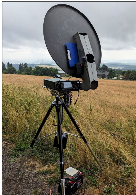
The big antenna (90 cm dish) of Walter's Station
