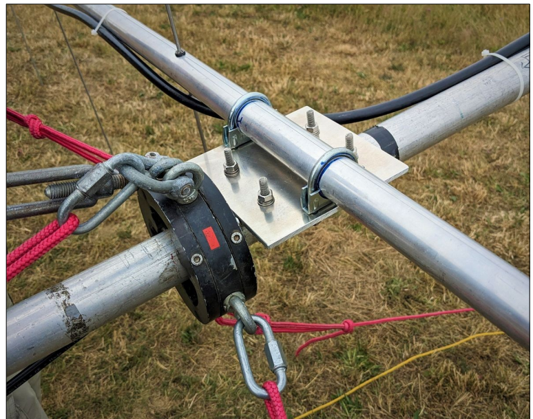
The M2 antennas have been equipped with modified mounting plates for easier installation
