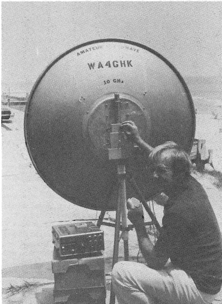
Fig. 6-9. WA4GHK sets the phase lock for a 10-GHz, 25-mile, over-water path. The signal will pass only a few feet above the water.
