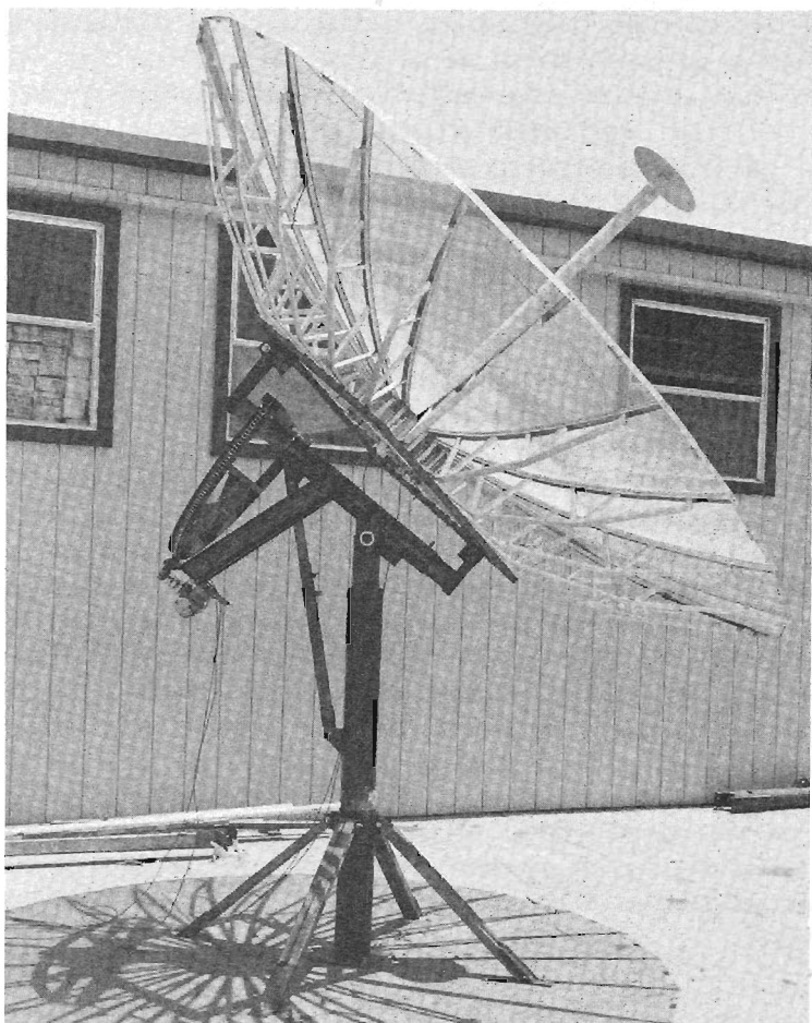
Fig. 12-6. The KLM 11-foot parabolic dish and motorized mount provides excellent performance for almost any area of the United States (courtesy KLM Electronics, Morgan Hill, California).
