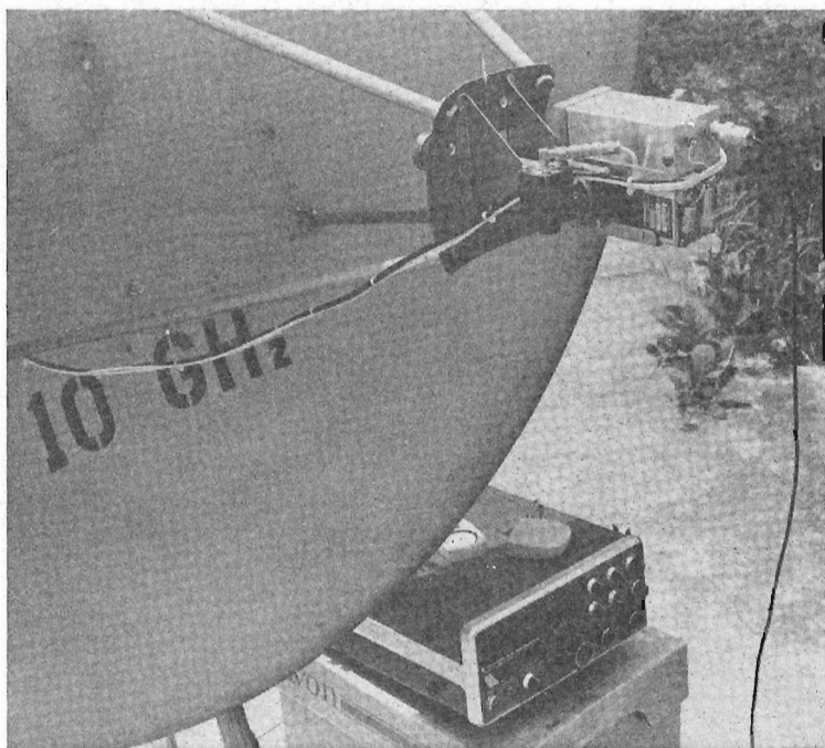
Fig. 6-8. The electronics of Fig. 6-7 seen from the opposite side. The i-f preamplifier is mounted atop the Gunnplexer. The Kenwood TS700A transceiver is the i-f receiver/transmitter.
