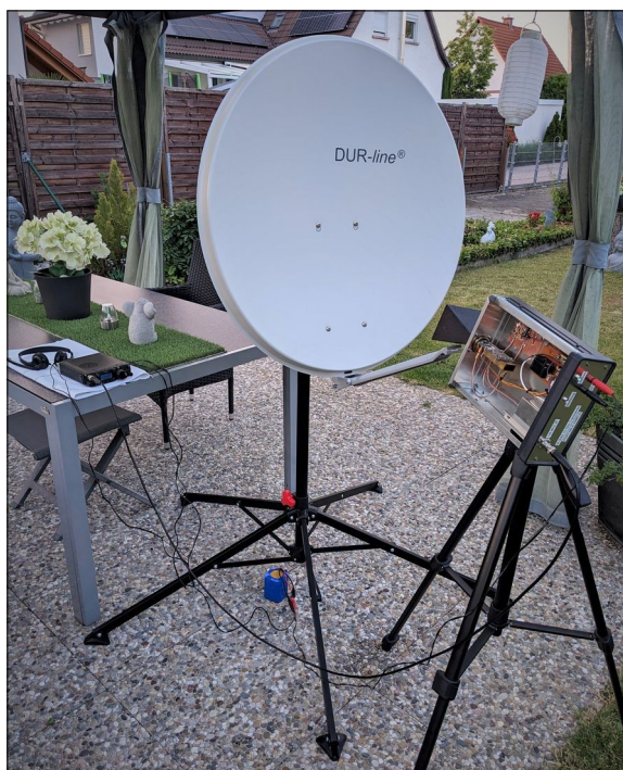
Yes, I am fully aware that a 16 dBD horn as feed under-illuminated this 75 cm offset dish!
