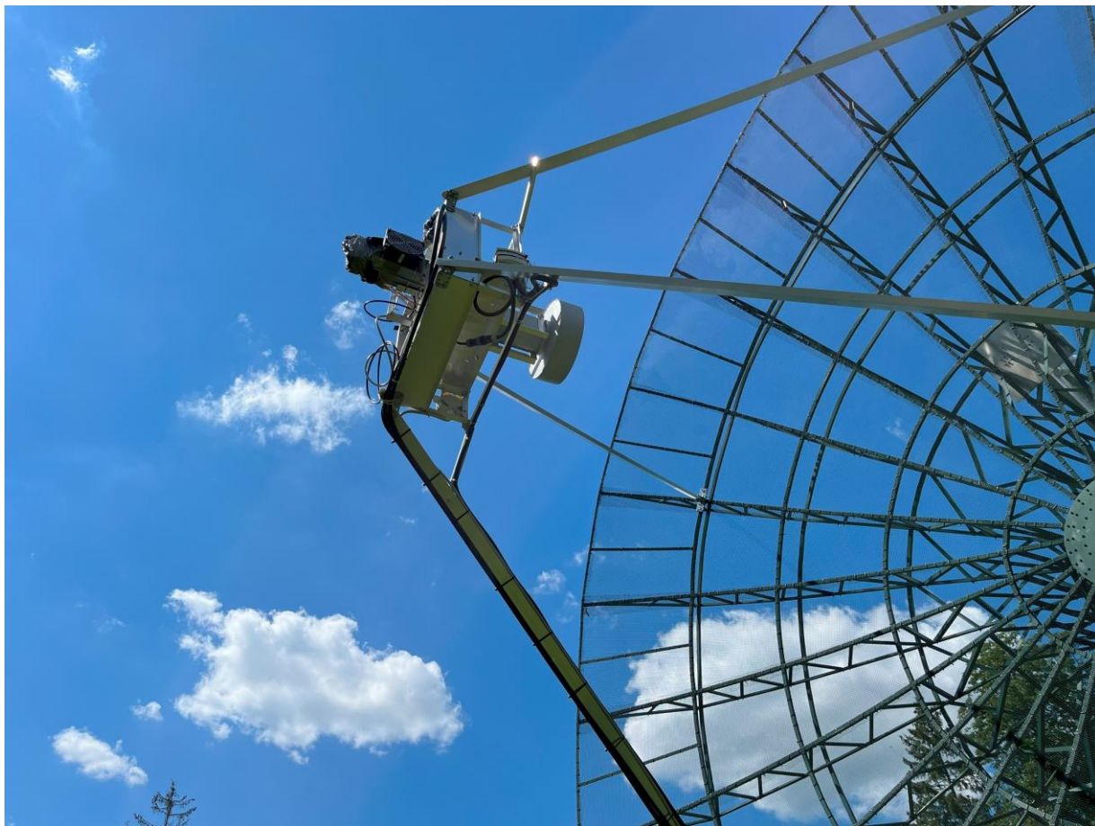
13 cm septum feed, relay box with LNA and 150W SSPA
