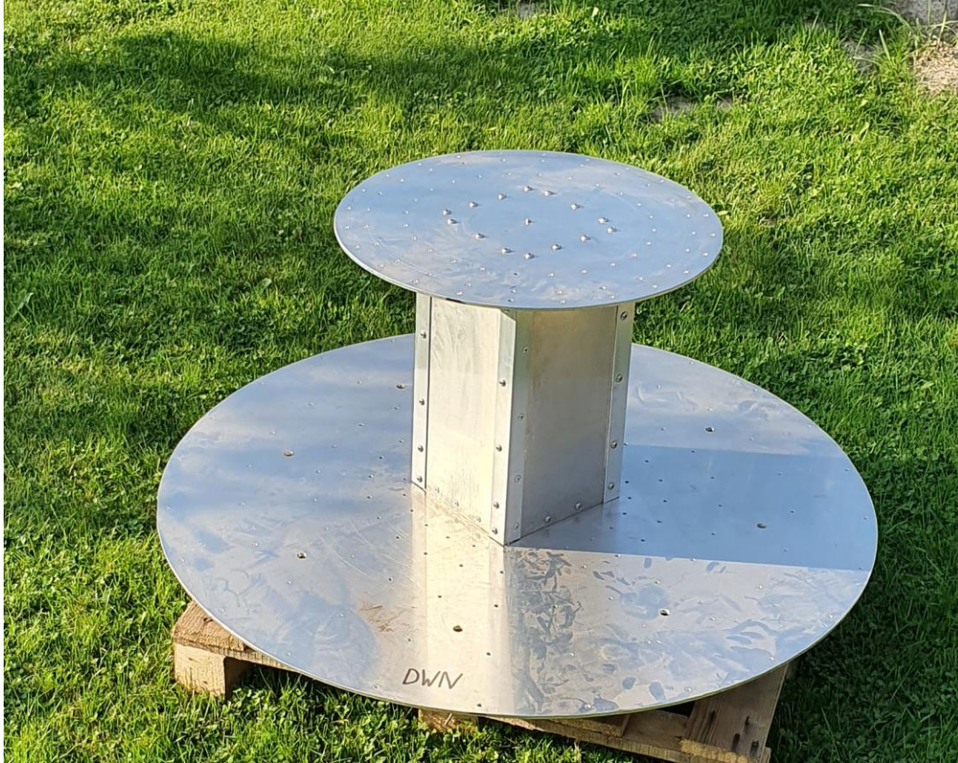
The HUB, central part of the dish. Aluminium plate 6mm thickness. Front side wheel 60cm diameter, back side wheel 100cm, distance between wheels 45cm.
