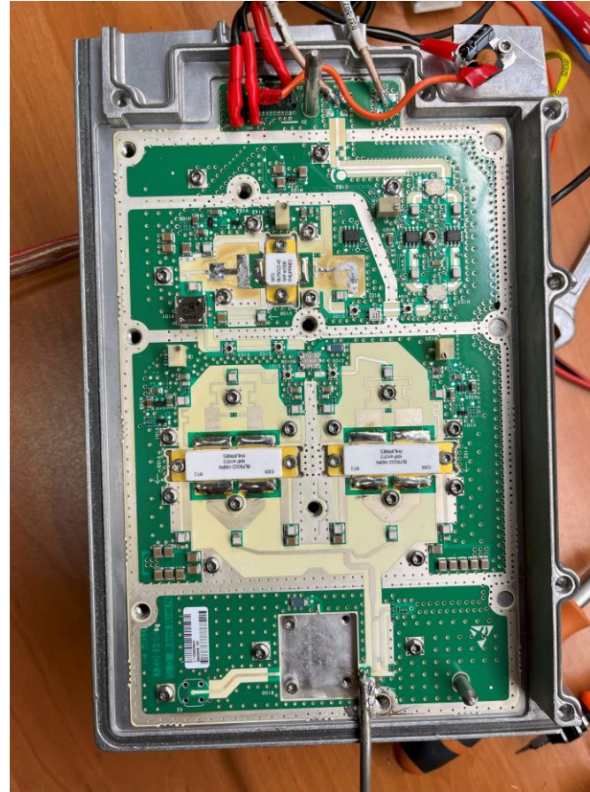
2 x BLF6G22-180PN UMTS SSPA surplus board. Surplus part, easy adaptation to use on 13cm.
