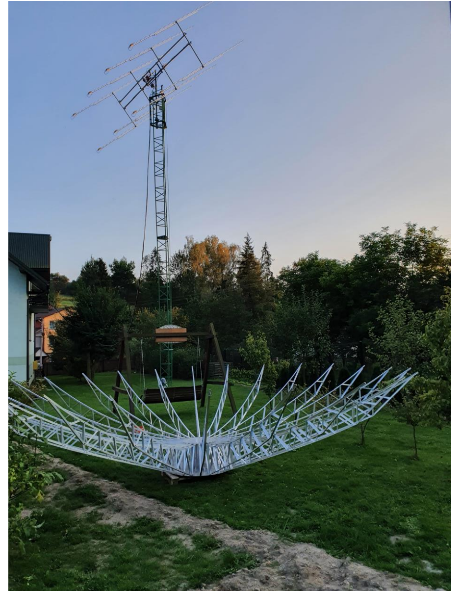
Pre-assembled 6.4m dish and set of 8 x 23 432MHz on the tower.
