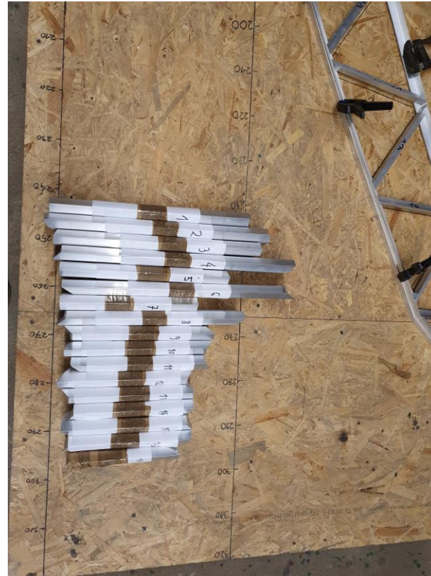
A set of already prepared elements for the ribs. All elements of aluminium angles 20x20x2mm.
