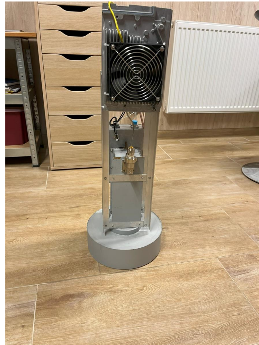
13 cm septum feed, relay box with LNA and 150W SSPA
