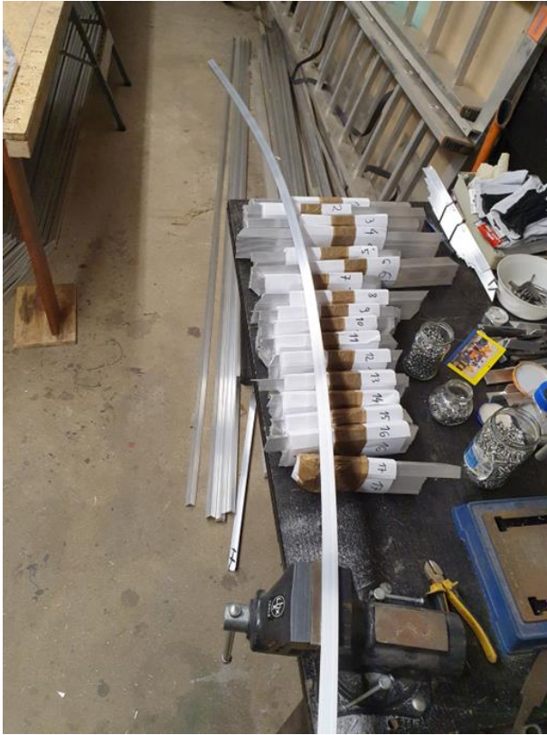
Pre-bent aluminium angle, by hand...
