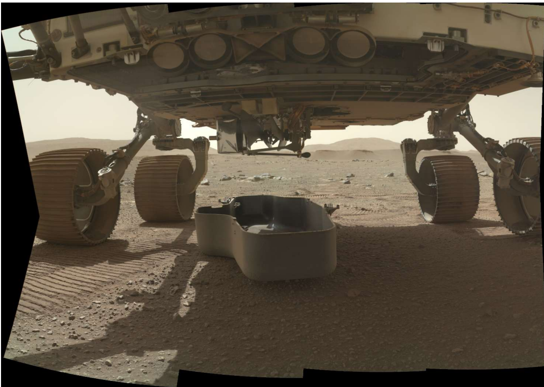
Debris Shield on Mars (with a little dirt in it)
