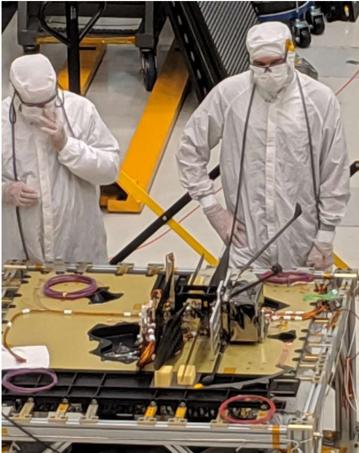
Landing Gear being folded
