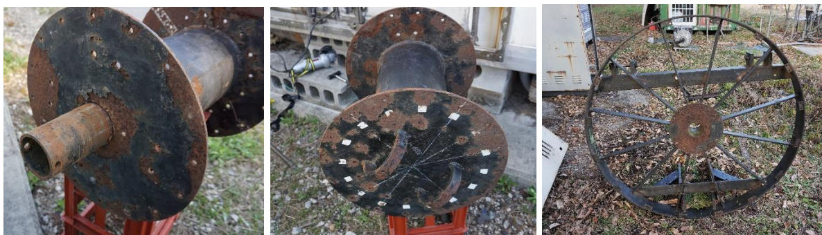
Spool (Hub), center of 16 trusses
