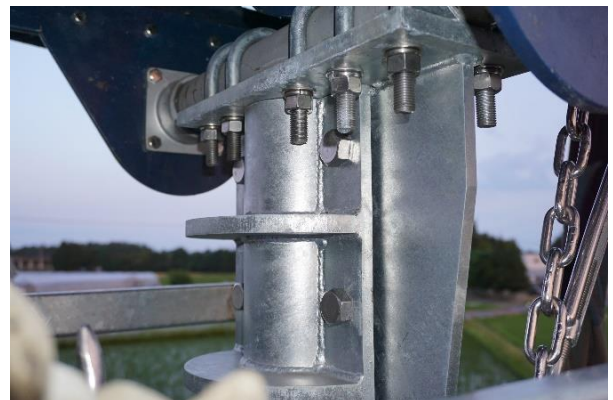
Bearing shaft 60 mm, Axis is solid steel rod 75 mm. Vertical rotary mast is 90 mm dia. solid shaft.
