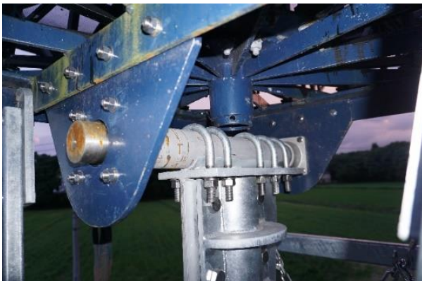
Bearing shaft 60 mm, Axis is solid steel rod 75 mm. Vertical rotary mast is 90 mm dia. solid shaft.
