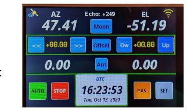
TFT 480x320 = 153,600 pixels Color Touch screen, no push buttons **32bit Dual core 240Mhz CPU up to16MB flash data memory**
