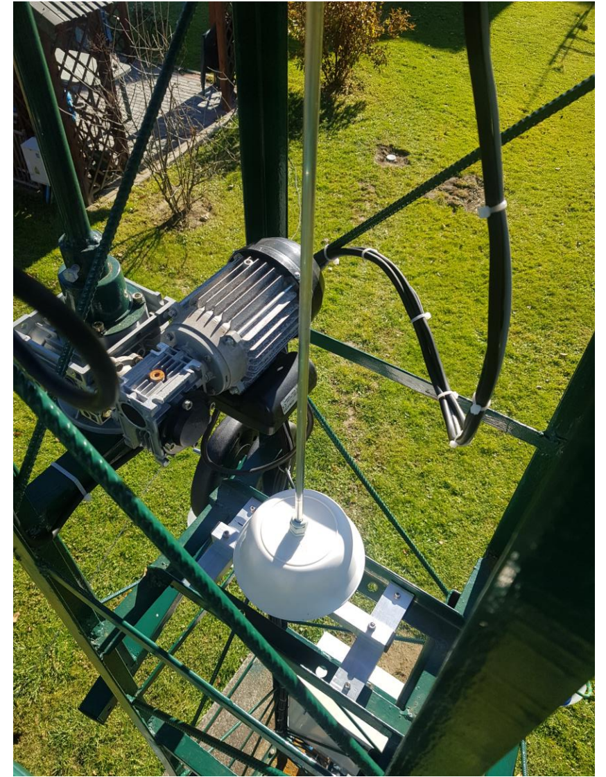
On the left AZ drive, 230V AC 180W engine with gear ratio 1:1200. On the right absolute encoder HH-12 enclosure.
