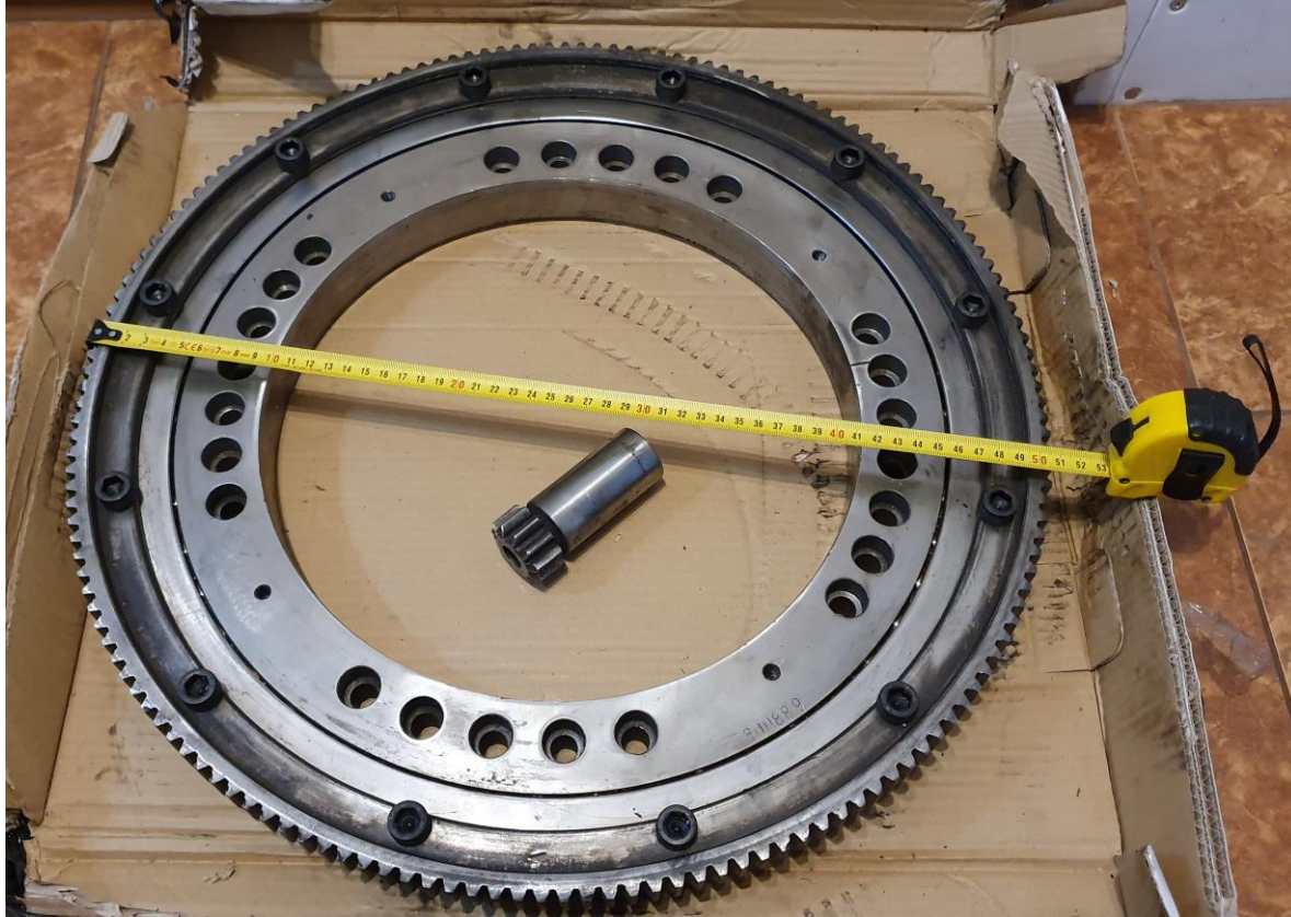
Mini crane main bearing, surplus part obtained from internet junk shop. Bearing with a diameter of 51cm. Load capacity several ton...
