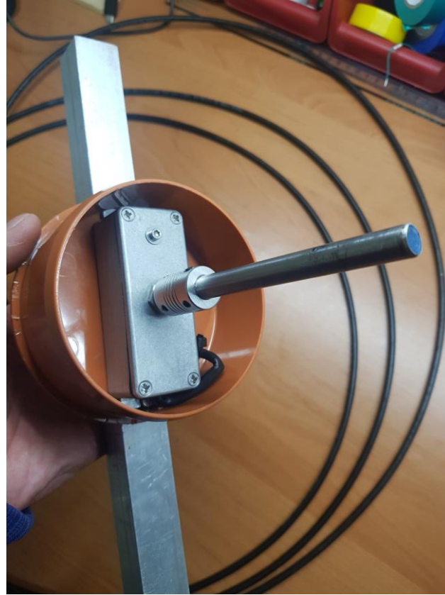
AZ reading, absolute encoder HH-12 DF1SR
