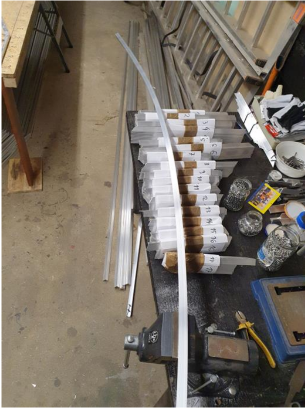
Pre-bent aluminium angle, by hand...
