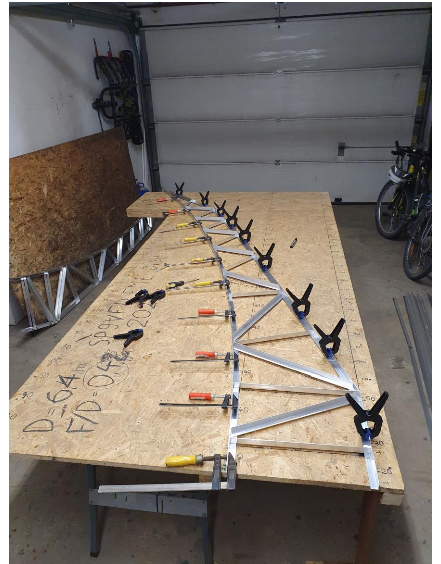
Template for the production of ribs, also made of aluminium angles 20x20x2mm.
