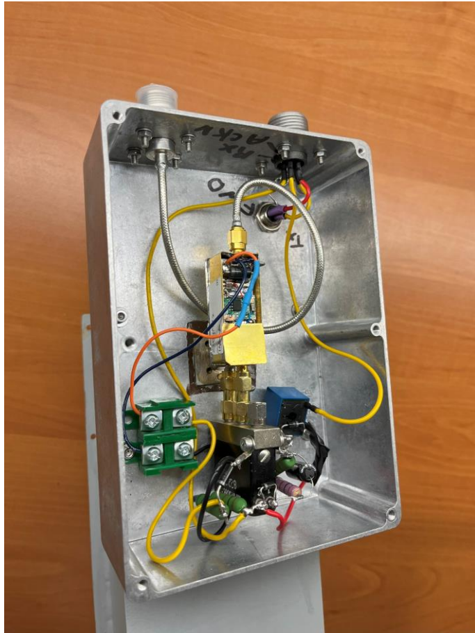
13cm WA6PY LNA 0.3dB NF 33dB gain. Aluminium enclosure with protection SMA relay.
