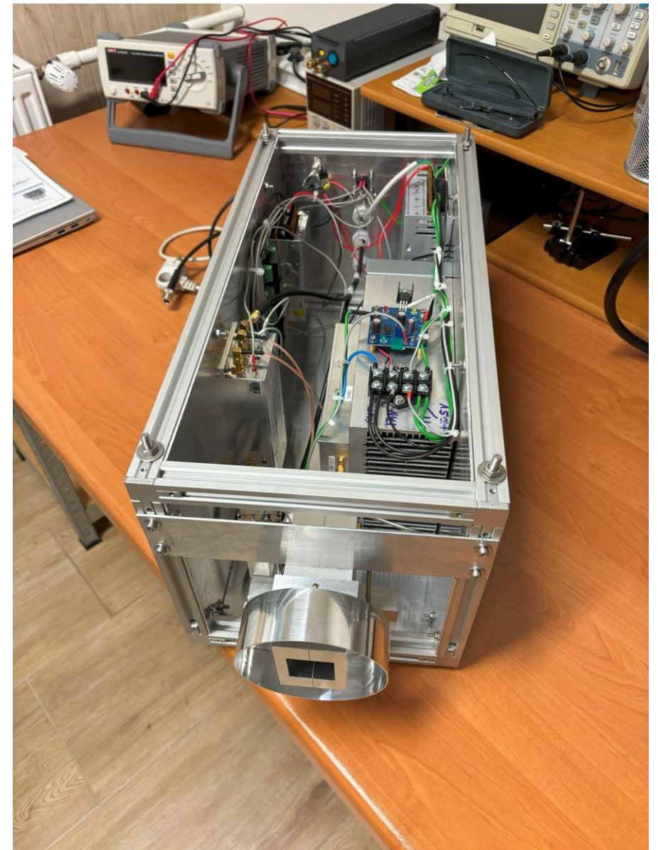
RFDdesign septum feed, DU3T LNA 0.68dB NF 26dB gain, MKU 57 G4 Kuhne TRV, 40W PA3DZL SSPA
