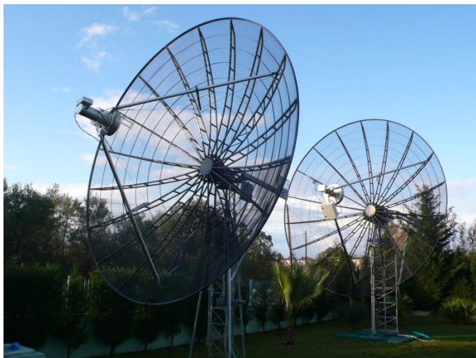
Jimmy, SV1BTR, used this pair of 6.1-meter dishes on 23 cm (1296 MHz, left) and on 70 cm (432 MHz) / 13 cm (2.3 GHz). He also has a dish for higher-frequency microwave bands and an array of phased Yagis for 2 meters. (Photo by SV1BTR)
