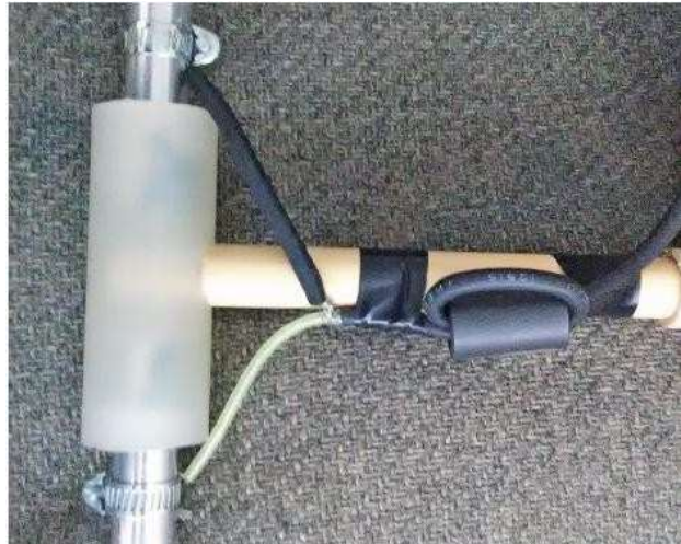
Figure 4.4.2: Radiation characteristics, blue line for metre waves, red line for decimetre waves Fig. 4.4.3. Detail of assembly and connection of the dipole
