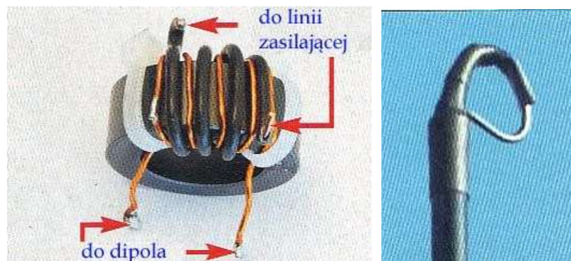
Fig. 1.2.2.3. Method of making the matching transformer
