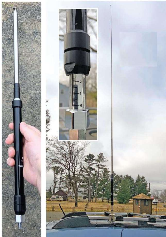
Photo A.1. MFJ-1898 is 55 cm long when the components are fully inserted (left)
