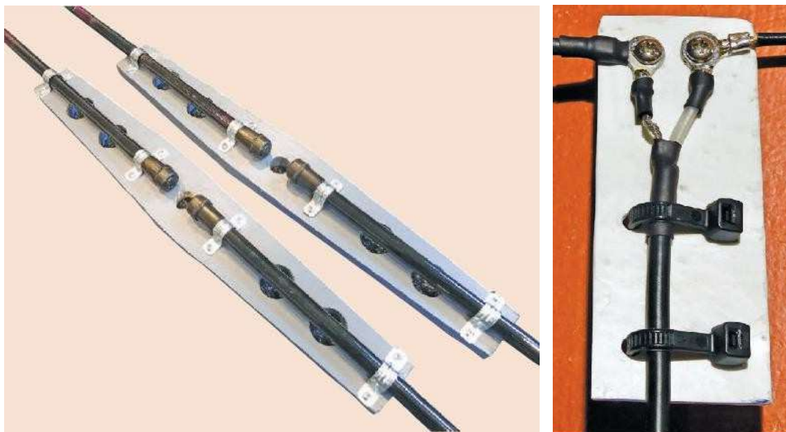
Photo 1.1.4.2. Fixing of rod ends on boards Photo 1.1.4.3. Method of making clamps
