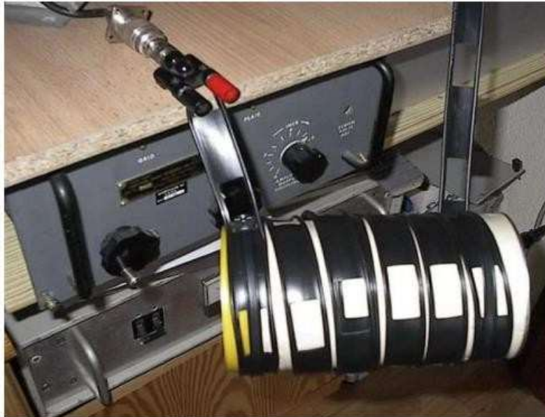
Photo 1.1.2.2. Flat cable symmetrizer. In the picture connected to the measuring system
