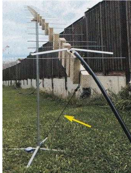
Fig. 4.1.4. Finished antenna and direction setting method
