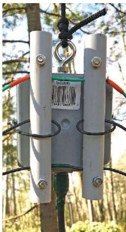
Photo 1.1.5.3. Junction box with symmetriser and two PVC struts
