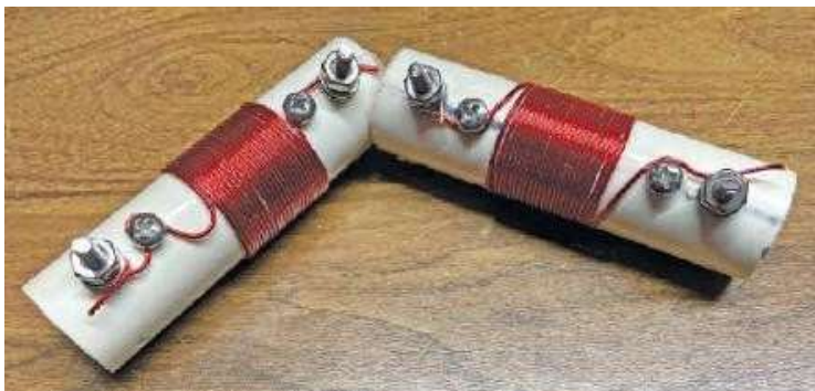
Photo 1.2.7.3. Extension coils for the 30 m band before they are impregnated and installed
