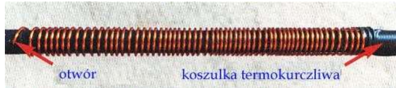
Fig. 1.2.2 Coil and supply assembly. On the left you can see the opening to the inside of the tube, and on the left the method of protection with heat shrink sleeve.
