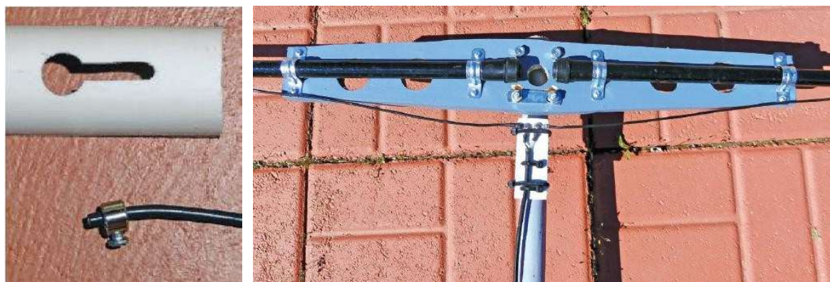
Photo 1.1.4.4. Insulators connecting the ends of the radiator and reflector Photo 1.1.4.5. Connection of the radiator
