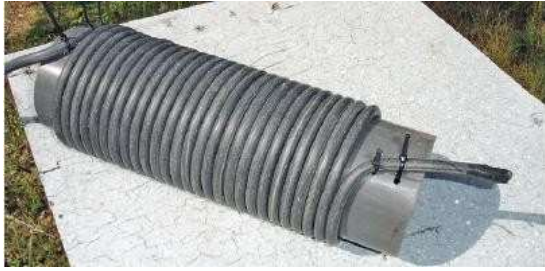
Photo 1.2.9.2 The choke consists of 27 coils of coaxial cable wound on a PVC tube with a diameter of ~11 cm
