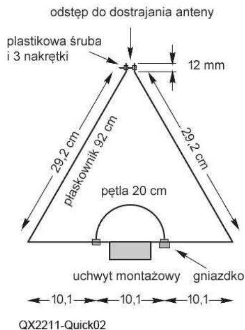
Photo 4.3.1. Triangular 2 m loop antenna with feed loop Fig. 4.3.2. Antenna dimensions
