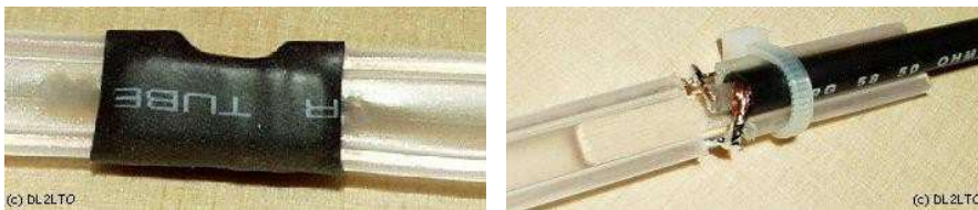
Fig. 4.2.7. Possible way of securing the gap with a heat-shrinkable jacket Fig. 4.2.8. Possible way of securing the cable at the end of the antenna.
