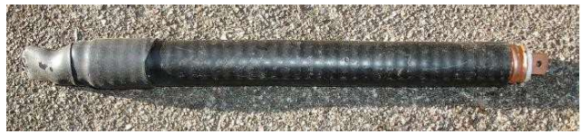
Photo 1.2.9.2 The choke consists of 27 coils of coaxial cable wound on a PVC tube with a diameter of ~11 cm
