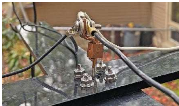
Photo 1.2.7.5. Connection of the upper dipole arms to the extended centre contact of the socket using a metal clamp
