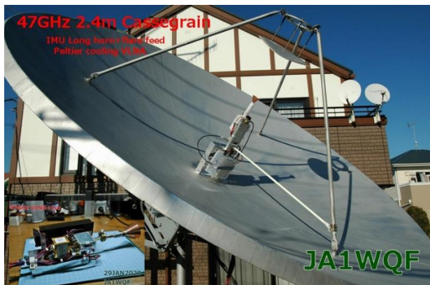
JA1WQF's 2.4 m dish with Cassegrain feed
