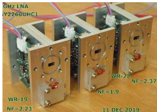
Three 47 GHz 1.9 dB NF LNAs
