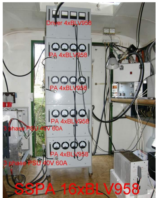
SP6JLW's "small" 1.2 kW SSPA for 23 cm
