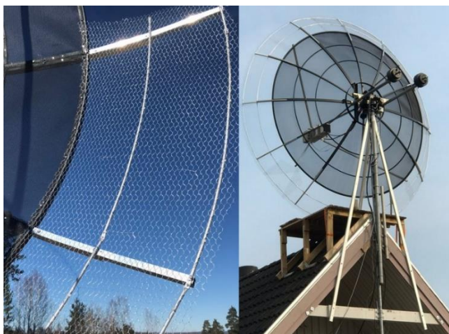
Details of SM4GGC's extension of his dish to 3.9 m
