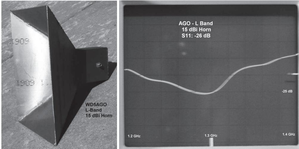
Appendances: Optimum 15 dBi pyramidal standard gain horn using smaller rectangular (2.6 x 5.6) waveguide, which cutoff is around 1.1 GHz (TE<sub>10</sub>). 6061 Al all welded construction. This waveguide size (6 inches long) as shown above provided one of the better broad band return loss of the transitions tested. This illustrates that a variety of waveguide sizes from 5.6 to 8 inches wide can be tuned to work all measured better than -18 dB return loss.
