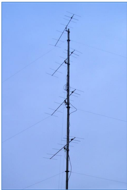
4 x 7 element fixed direction North F and South UK
