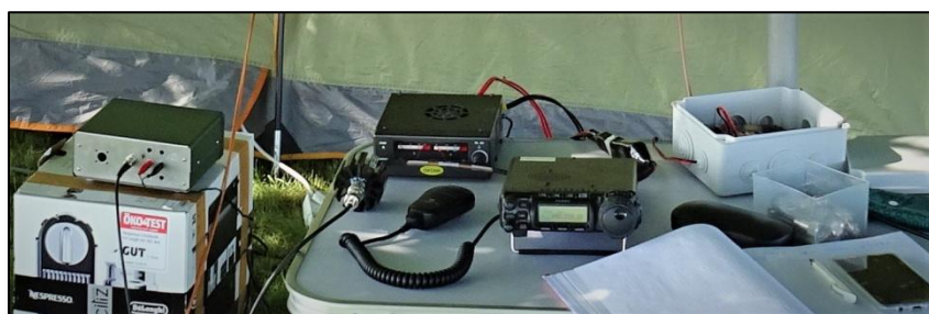
On the left: Box with 106,5 MHz PLL LO and 10 MHz OCXO for 10 GHz On the right: Yaesu FT857 and LZ5HP Transverter for 2,3 GHz *
