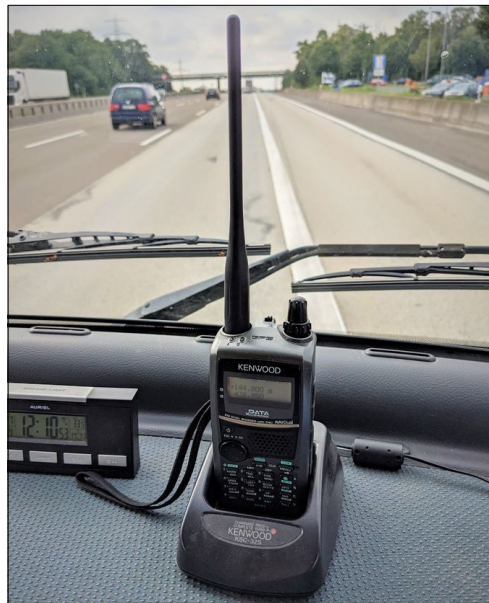
The Kenwood handheld TH-D72E was used as 5 Watt APRS beacon
