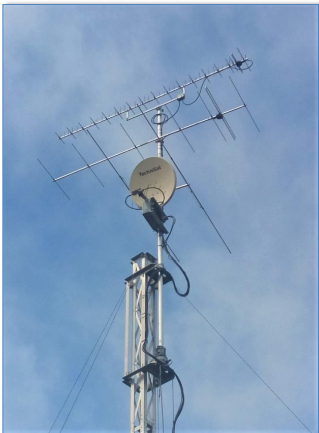
6m/2m/70cm yagis and the "small" 65 cm dish for 6cm/3cm
