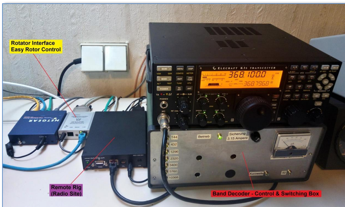
Access to the transceiver by inhouse remote (via LAN) at the radio site
